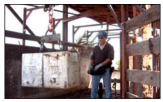
An Inspector using 1,000 pound test weights to check the accuracy of a cattle scale.
