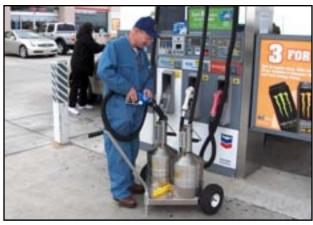
Liquid dispensing meters, such as gasoline pumps, are tested using standard volume containers called provers.
