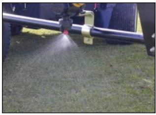
Worn nozzle tips cause higher application rates and changes in the spray pattern.
