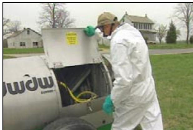
**When repairing contaminated equipment, wear the same safety equipment as would be required to apply the pesticide.**
